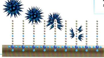
As the protective coating dries, millions of positively-charged microscopic "spikes" form and extend from the surface.
